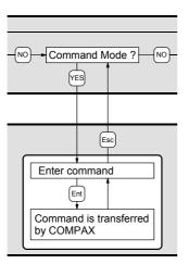
Once you have transmitted the command using "Ent", this command reappears in the display and it can be modified and transmitted again.
